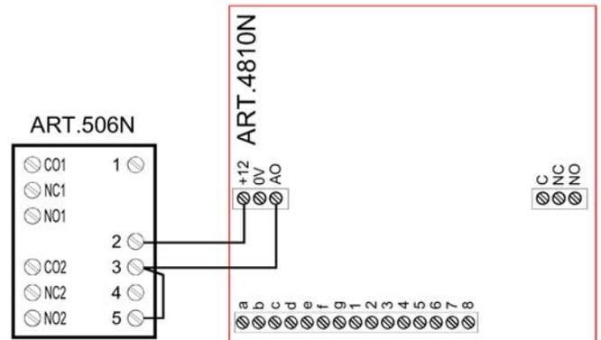
**AUXILIARY 1 INPUT, TRIGGERS AUXILIARY OUTPUT (AO)**
