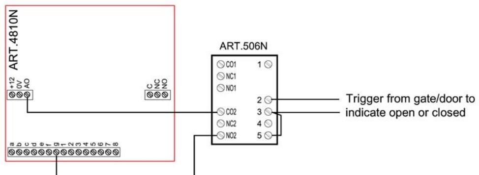
**NOTE: WHEN USING THE AO OUTPUT FOR STATUS INDICATION IT CAN NOT BE USED AS AN OUTPUT FOR ANYTHING ELSE.**
