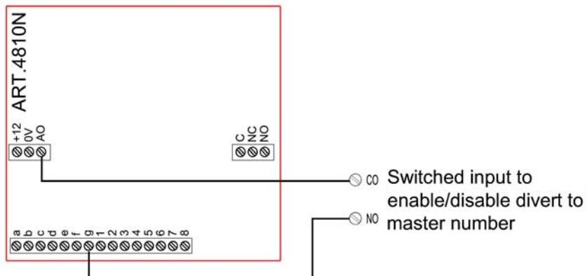
**NOTE: WHEN USING THE AO OUTPUT FOR DIVERT TRIGGER IT CAN NOT BE USED AS AN OUTPUT FOR ANYTHING ELSE.**
