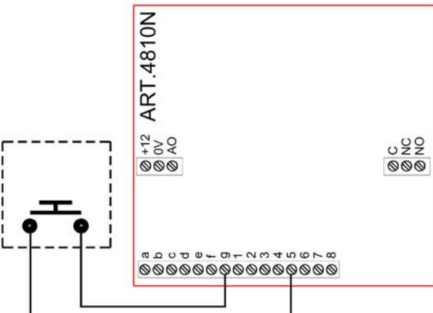
**AUXILIARY 2 INPUT, SENDS A SMS MESSAGE TO THE MASTER TELEPHONE NUMBER**
