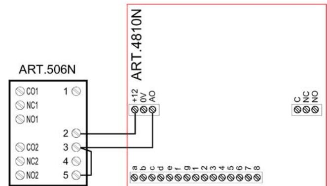
**AUXILIARY 1 INPUT, TRIGGERS AUXILIARY OUTPUT (AO)**
