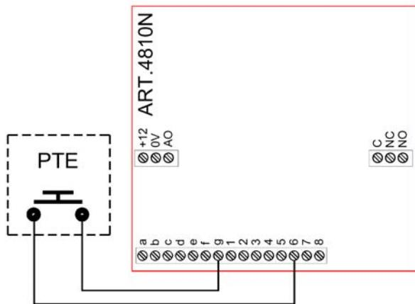
**AUXILIARY OUTPUT (OPEN COLLECTOR), TRIGGERS WHEN g & 5 ARE SHORTED**
